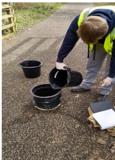
Plate 6.3-Infiltration test set up
