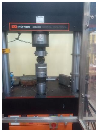
Plate 6.1-ITS and stiffness test set up on Instron machine
